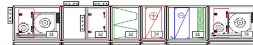
KS7- MIXED AIR AIR CONDITIONING PLANT Aspirator Cell - Ventilator Cell - Heating Cell - Cooling Cell Bag Filter Cell - Mixing Cell
