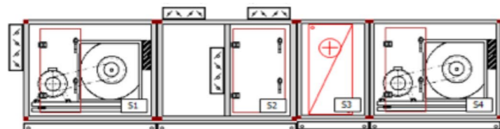
KS5 MIXED AIR AIR CONDITIONING PLANT Aspirator Cell - Ventilator Cell Heating Cell - Mixing Cell
